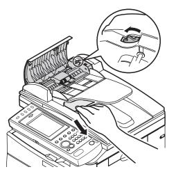
**3** Close the ADF cover. Make sure both sides are snapped down securely.
