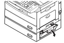
2 If paper is jammed in the paper supply area, remove the jammed paper.
