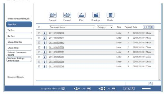
If you save the documents scanned on the machine in a user box on the Message Board, you can transmit the data for the scanned documents via e-mail and fax. You can also save received faxes in the shared reception box and user box without printing them. You can conserve paper by viewing documents on a PC rather than printing them.
