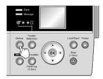
Roll paper is fed to the specified cut position and then automatically stopped.
