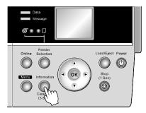
Press the Information button to display the Maintenance Cartridge capacity and remaining ink levels, as well as information on the loaded paper and the printer. Press the Information button repeatedly to change the information displayed. (→P.66)
