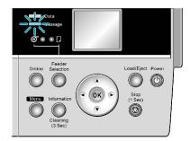
If the Data lamp is flashing, the printer is receiving a print job. Turn off the printer only after printing is finished.
