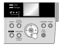
The printer returns to the mode before replacement of the Maintenance Cartridge. If a message is displayed advising you to replace the Maintenance Cartridge, printing is not possible. Make sure that the Maintenance Cartridge is installed correctly.
