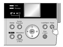
**2.** The printer goes online in preparation for printing after startup, and the Online lamp and paper source section lamp remain lit.
