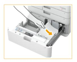
1 Load the paper stack with the print side face up, and against the right side wall of the paper drawer.
