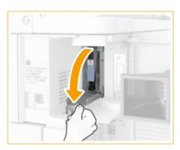
3 Hold the handle on the hard disk holder and remove the holder.
