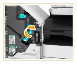
4 If paper comes out of the outlet of the main tray, gently pull the paper out in the direction of the arrow.
