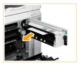
2 If paper is jammed in the lower area, gently pull it out in the direction of the arrow.
