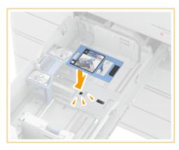
3 Attach the Envelope Feeder Attachment A by aligning the protruding areas of the Envelope Feeder Attachment A with the holes on paper receptor located on the bottom of the paper drawer.
