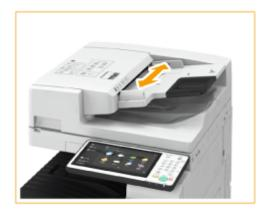
• When placing large-sized originals, pull out the original supply tray extension and original output tray extension to prevent them from dropping over the edge of the feeder.
