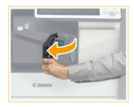
3 Hold the lever ( 6), and slide the inner finisher to the left.
