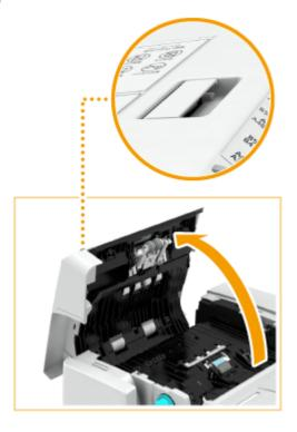
**3** Clean the rollers inside the feeder cover.
