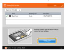
• If you press <Remove Toner Cartridges>, the replacement cover (small cover) opens automatically.
