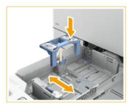
2 Adjust the left guide of paper drawer 1, and attach the Envelope Feeder Attachment B to the left guide.
