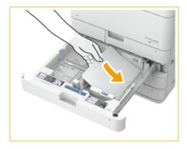
• Load the tab paper with the tabs on the left side.
