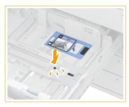
2 Attach the Envelope Feeder Attachment A by aligning the protruding areas of the Envelope Feeder Attachment A with the holes on paper receptor located on the bottom of the paper drawer.
