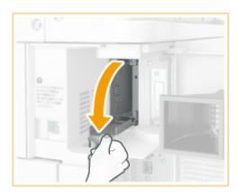
3 Hold the handle on the hard disk holder and being careful of the orientation, insert the holder.
