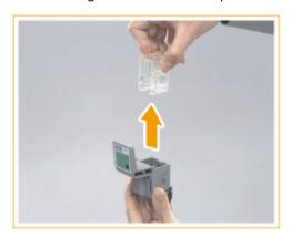
5 Remove the new staple cartridge from its box.
