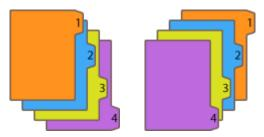
When you load tab paper into the paper drawer 2, load right order tab paper face up with the tabs on the left side. For the reverse order tab paper, load face up with the tabs on the left side in the same printing order as the right order tab paper.
