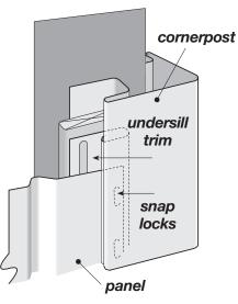
**NOTE:** The cutting and supporting procedure described above is also used when fitting panels into inside cornerposts.
