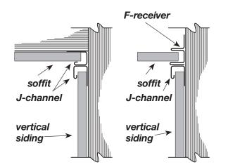
Install inverted J-channel along the top of the wall, under the eave. Here again, leave a 1/4" gap between Jchannel and cornerposts. Overlap J-channels 3/4" to allow for expansion. When positioning the upper Jchannel, be sure to allow for expansion of the siding panel. In most cases, position the J-channel at a point equal to the length of the panel plus 5/8" (1/4" for upper expansion and 3/8" for lower expansion).
