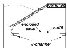
The procedure used to install soffit over an enclosed eave is almost identical to that used for an open eave. The major difference is the installation of the J-channel. Determine the method you'll use to install soffit at the fascia board (see figures 8 and 9). When installing J-channel at either the wall or the fascia board, nail the J-Channel every 12"-16".
