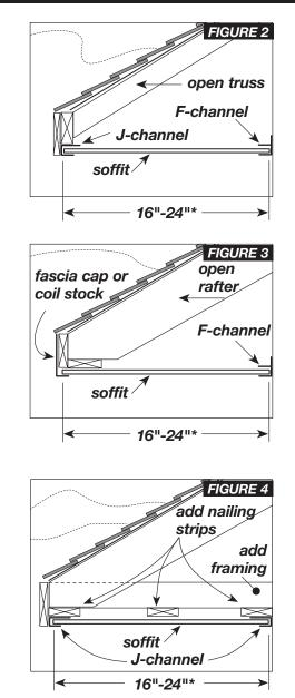
If no F-channel is available, J-channel can be modified to create F-channel. Simply cut slots (as shown in figure 5) in the nail flange area where it would be nailed to the
