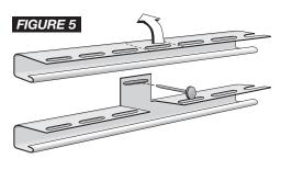
wall. After cutting the nail flange, bend the flange back and nail to the wall. When installing Beaded T2" panels, use 3/8" H-bar or 3/8" J-channel.
