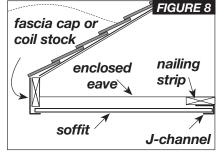
perforated soffit panels and the existing soffit doesn't have openings for ventilation, cut an adequate number of openings. Then complete the installation as described for open eaves.
