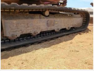
Right Side: Link Bushings / Drive Sprocket / Shoe Condition
