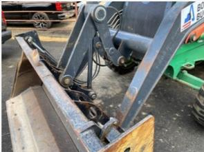
Tilt Linkage Pins & Bushings
