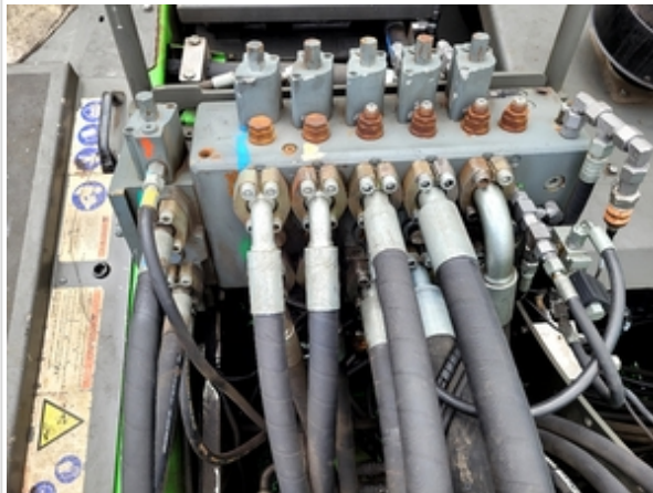
Main control valve is leak free and hoses to it are in good shape.
