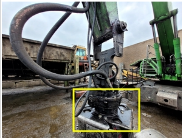
Surface wet of residual hydraulic oil
