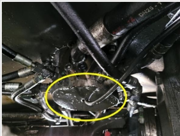
Minor hydraulic fluid seen at bottom of hydraulic swivel
