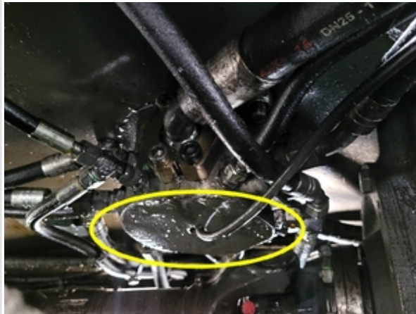
The circled area has minor hydraulic oil buildup. Minor active leak present at swivel.
