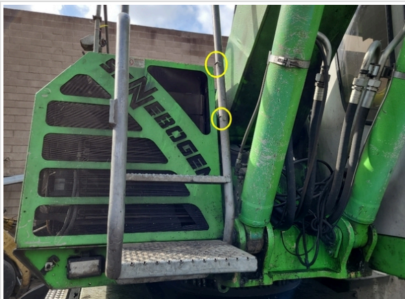
Steps Broken Off
