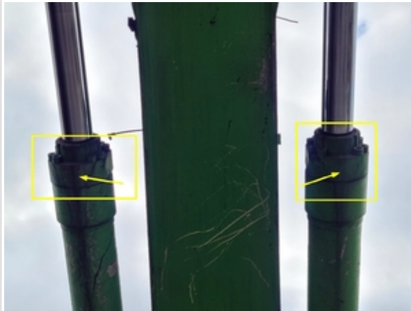
Could be old grease lyquifyin down cylinder from rod end.
