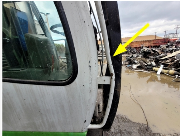
R/S Cab Exterior Handrail slightly bent.
