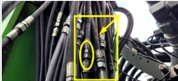
Circled area slightly leaking and pointed area shows hose surface rubbing
