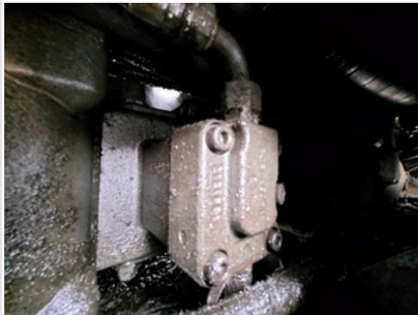
The circled area has minor hydraulic oil buildup. Minor active leak present at swivel.
