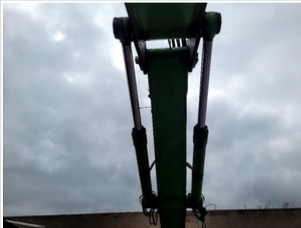
Could be old grease lyquifyin down cylinder from rod end.
