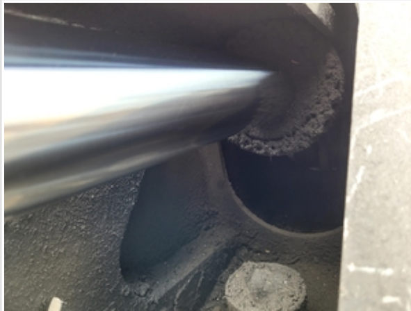
Circled area slightly leaking and pointed area shows hose surface rubbing
