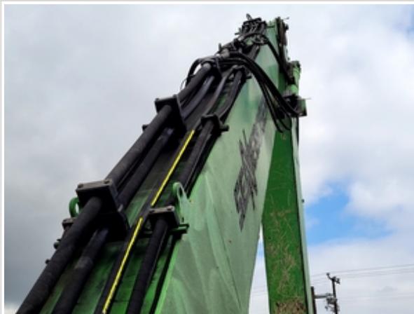
Highlighted Hose missing mounting brackets
