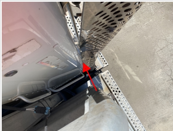
Exhaust shield damaged and pressed up against cab
