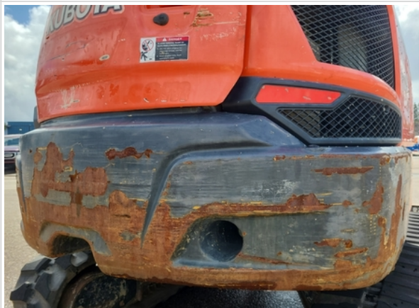
Normal wear and tear scuff marks and minor surface rust observed on counter weight
