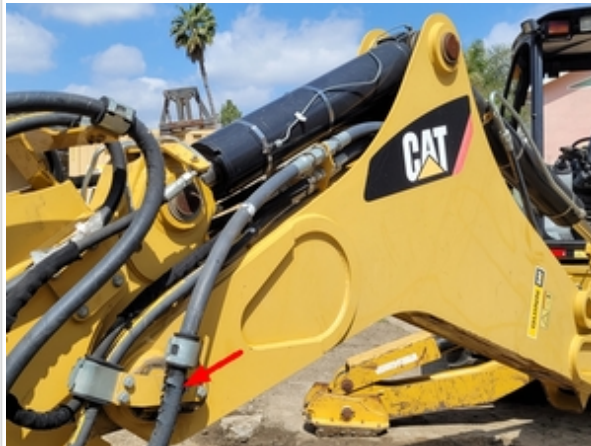
Hydraulic Hose exterior cracking
