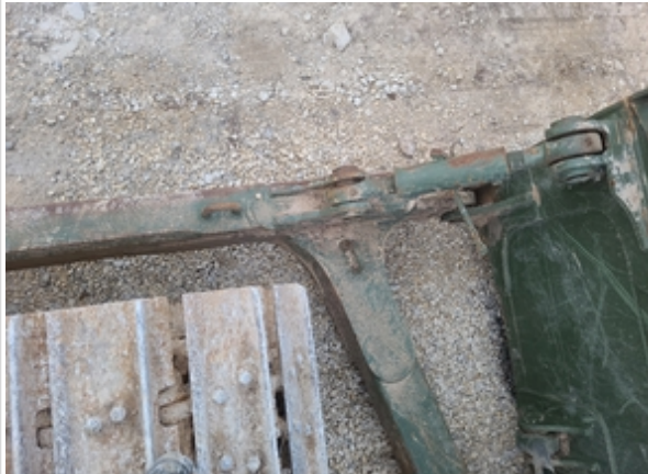
Left side blade bracket has improper retaining hardware
