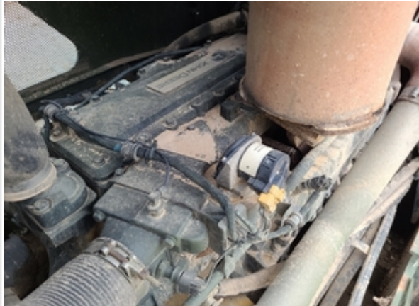
Minor engine oil leak at mounted seal
