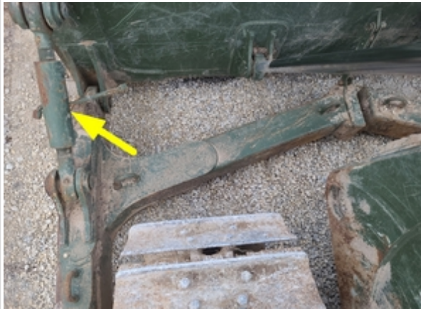
Left side blade bracket has improper retaining hardware
