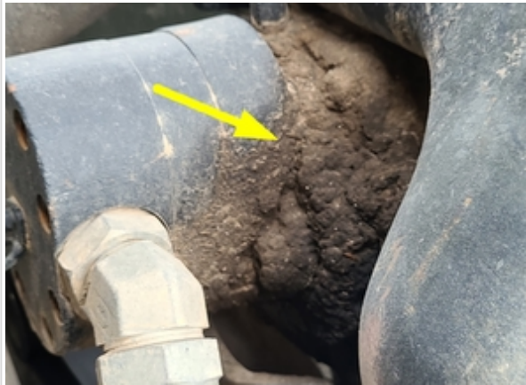
Minor engine oil leak at mounted seal
