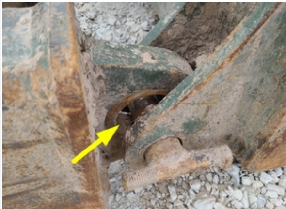
R/S Arm Bearing missing
