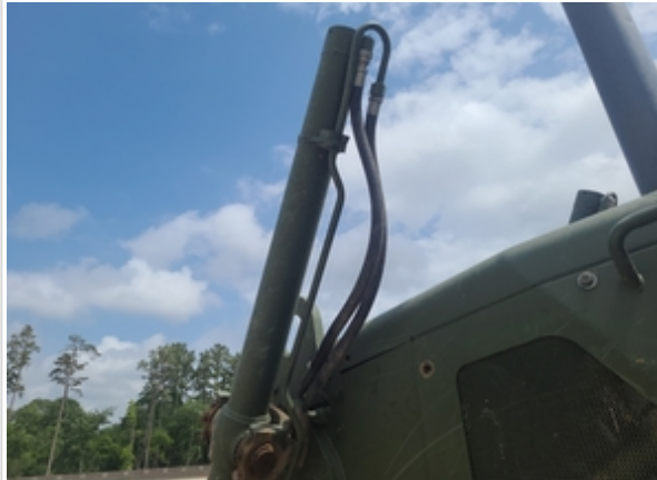
Possible small leak at hydraulic hose
