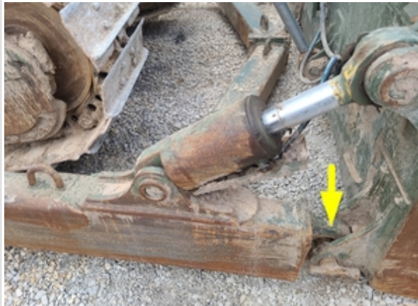
Right side arm retaining pin incorrect and bearing missing
