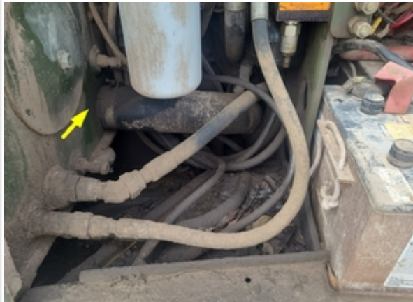
Possible small leak at hydraulic hose
