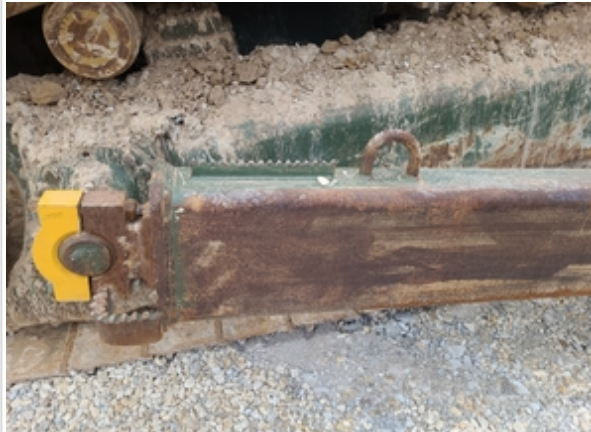
Right side arm retaining pin incorrect and bearing missing
