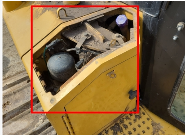
Top cover missing
