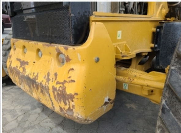
Bottom Powertrain Guard slightly bent
