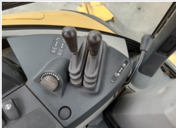
Control Grips have surface damage (cosmetic)
