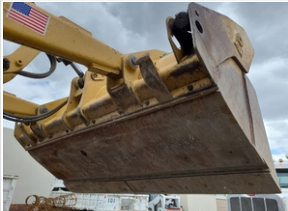
Additional section added to increase capacity capabilities on front bucket
