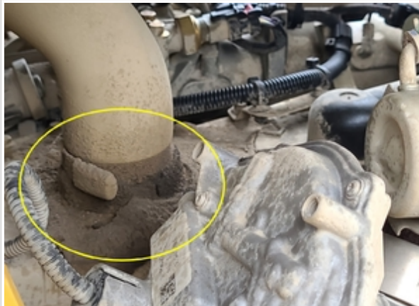
Residual Oil buildup
