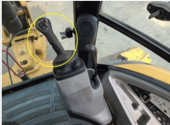
Control Grips have surface damage (cosmetic)
