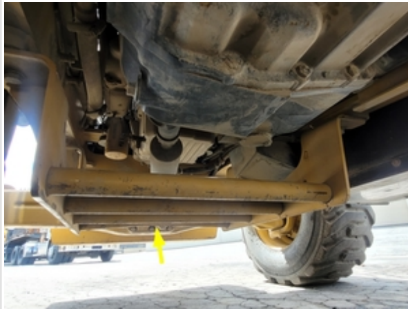
Bottom Powertrain Guard slightly bent
