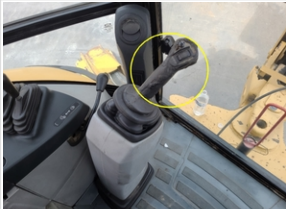
Control Grips have surface damage (cosmetic)
