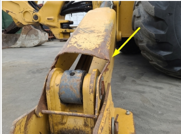
R/S Stabilizer Cylinder Shield bent
