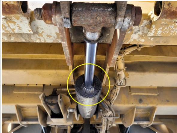
Cylinder has residual oil and may be leaking
