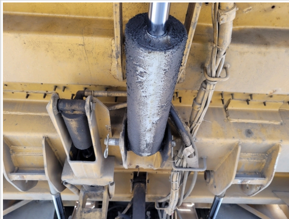
Cylinder has residual oil and may be leaking
