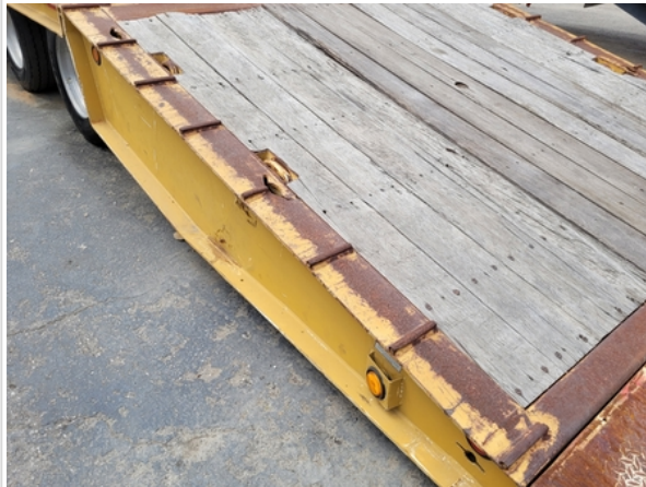
Floor board missing wood piece
