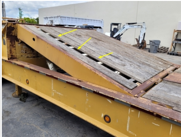
Floor board missing wood piece
