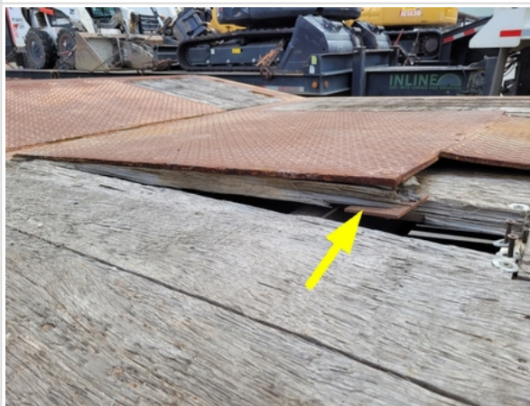
Wood damaged at front part of deck
