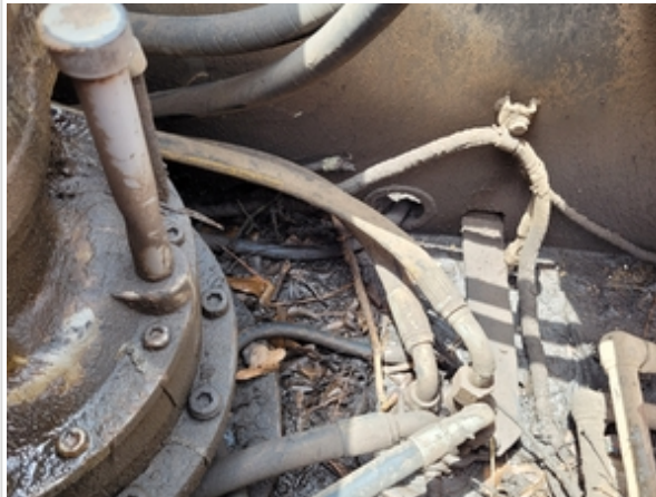
Hydraulic residual buildup around swing drive
