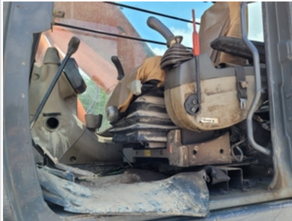
Hydraulic Pilot Control Hoses Leaking
