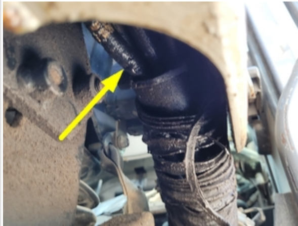
Hydraulic Pilot Control Hoses Leaking
