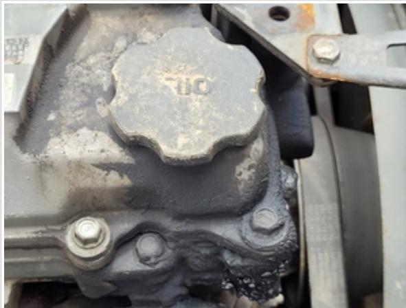
Active Engine Oil Leak
