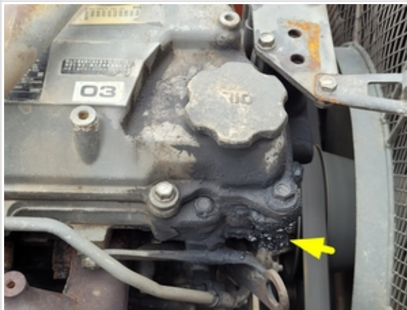
Active Engine Oil Leak
