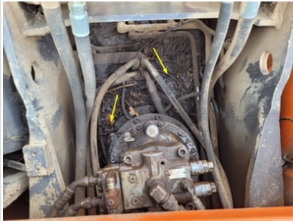
Hydraulic residual buildup around swing drive
