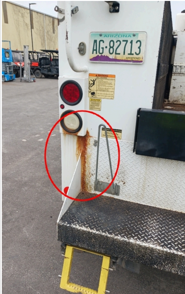
rusted area located on the left hand side of the box near the tailgate. the area is 17inches long
