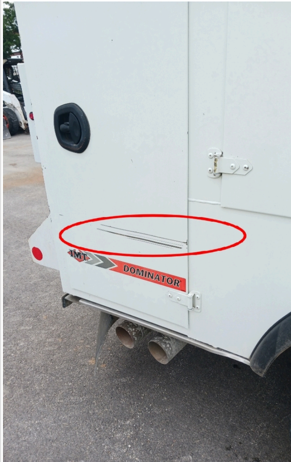
scratch on the right hand side box. 14inches long less than 1/4inch wide
