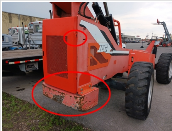
areas of scratches and rust
