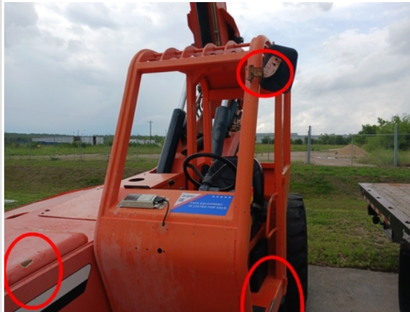
areas of rust and scrapes
