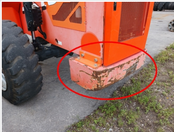
areas of scratches and rust
