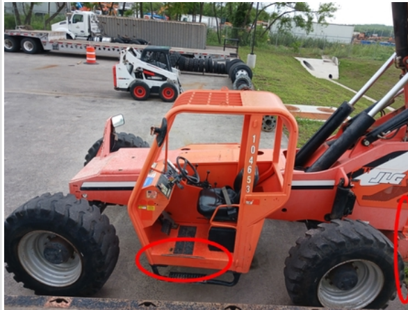
area of rust and missing paint
