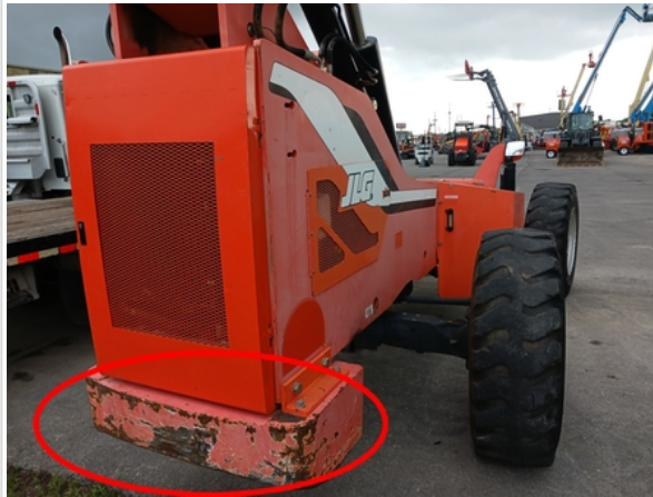
scratches and rust
