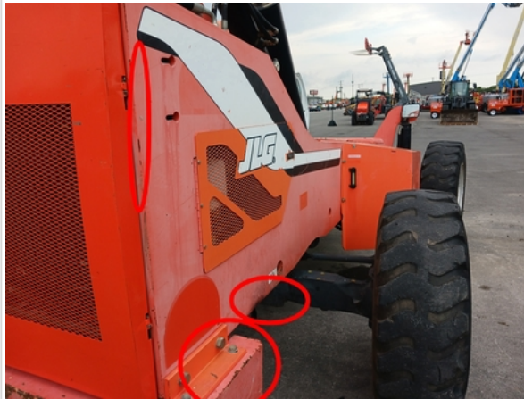
small amounts of rust
