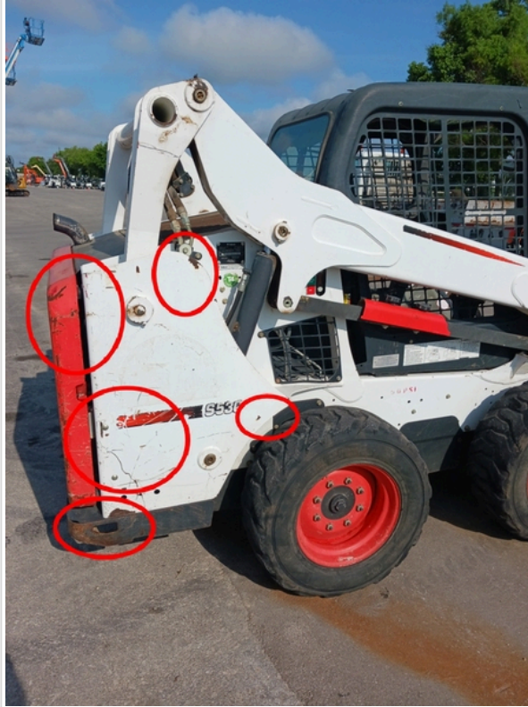
areas of rust and missing paint
