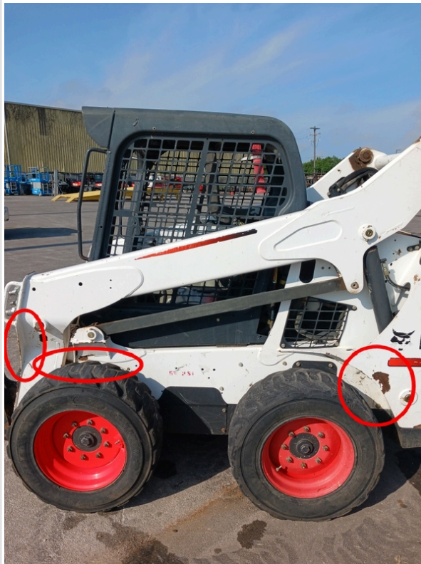
areas of rust and missing paint
