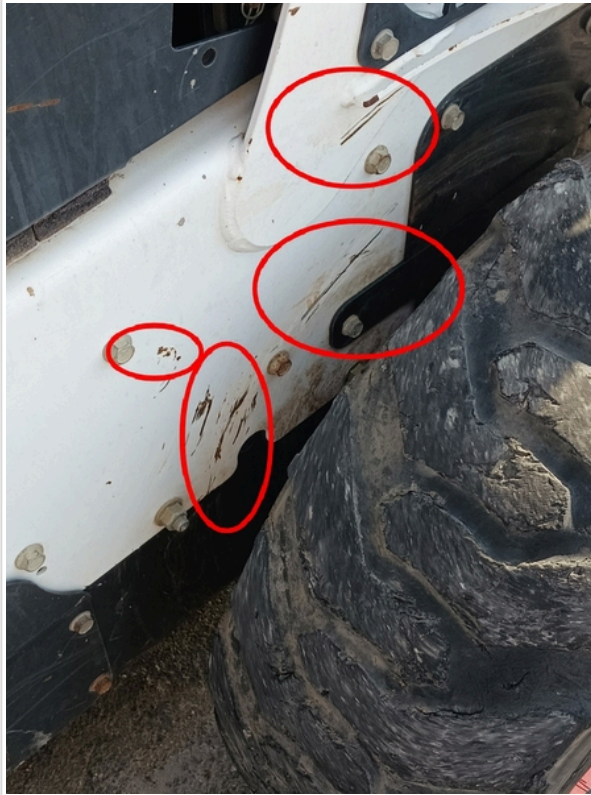
some rust and missing paint
