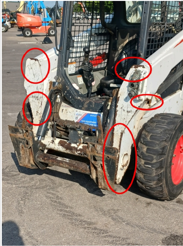
areas of rust and missing paint
