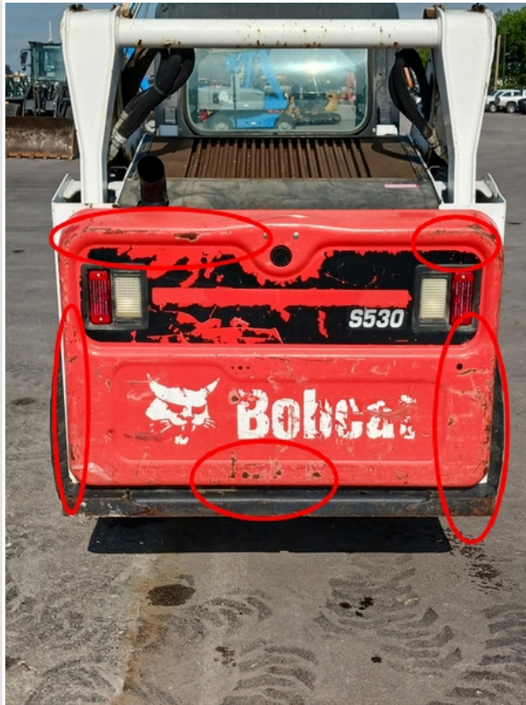
there are areas of rust and missing paint
