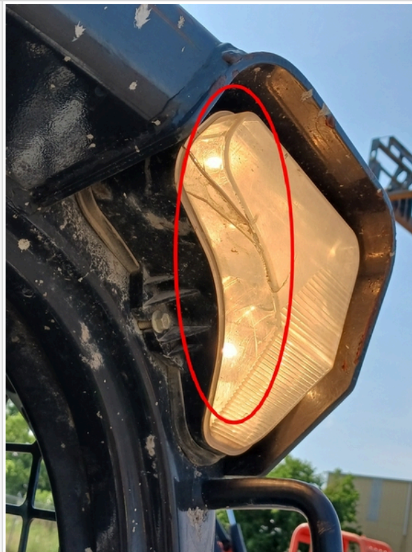
crack located under the light on the left hand side
