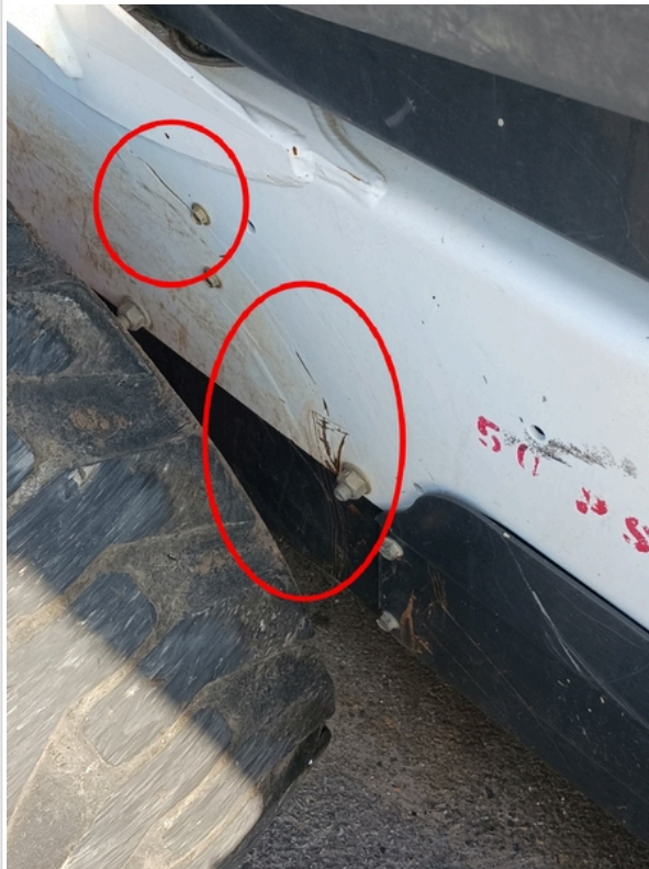
some rust and missing paint
