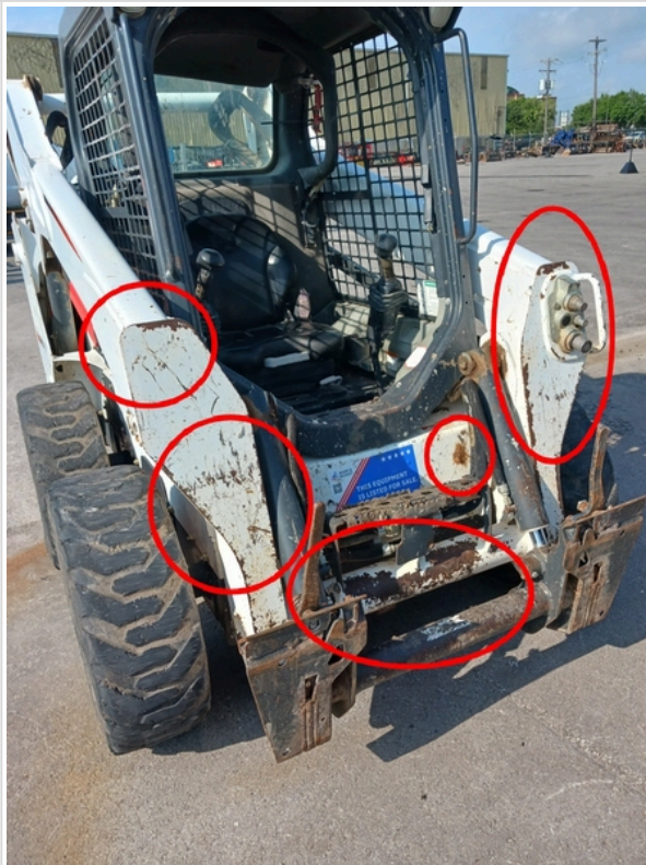
areas of rust and missing paint
