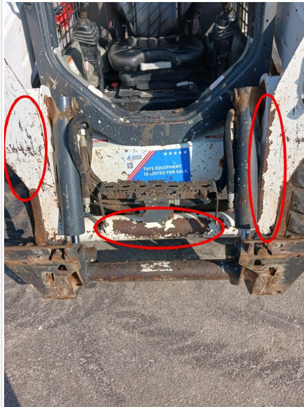
areas of rust and missing paint
