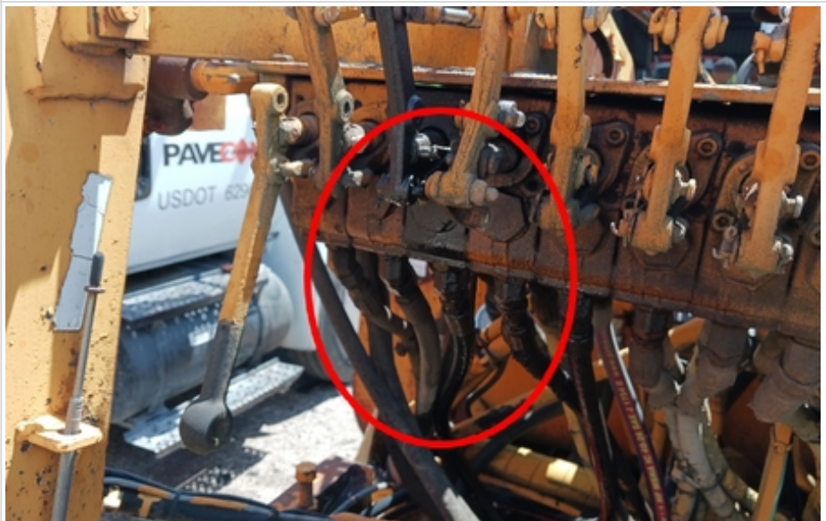
hydraulic fluid leaks out from the controls
