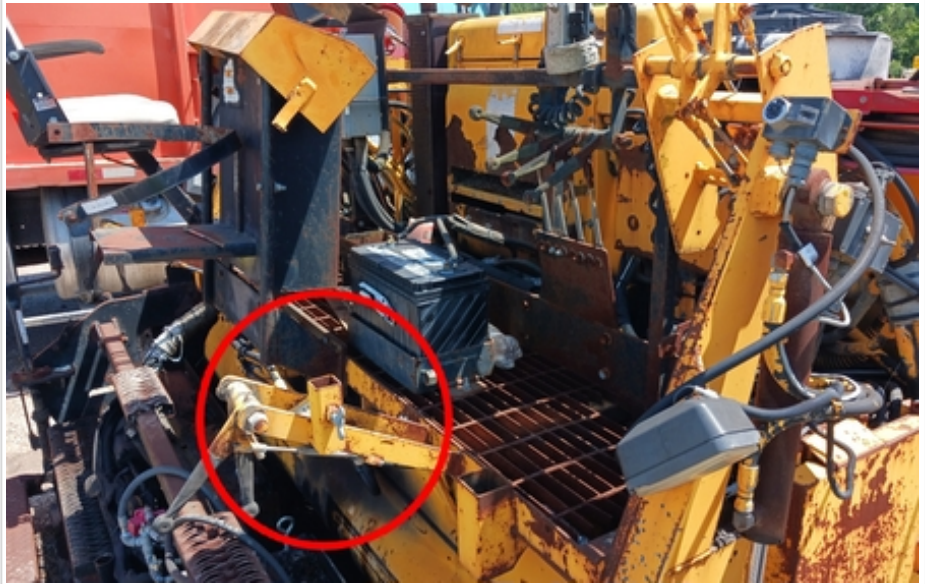
right side operators seat is missing
