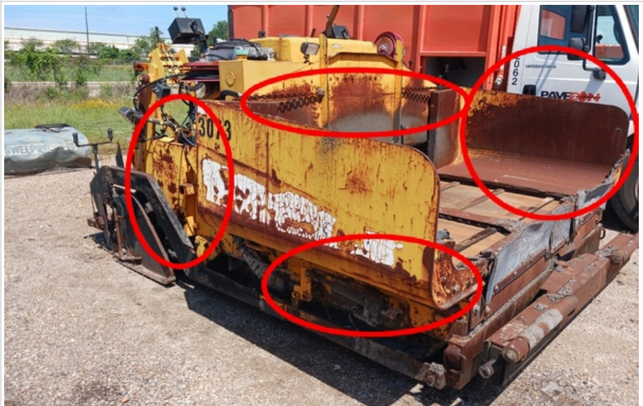
areas of rust
