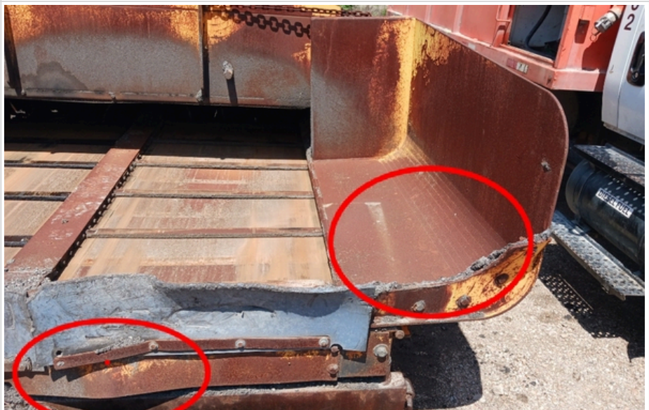
left hand hopper is missing rubber side wing and front strip is bent
