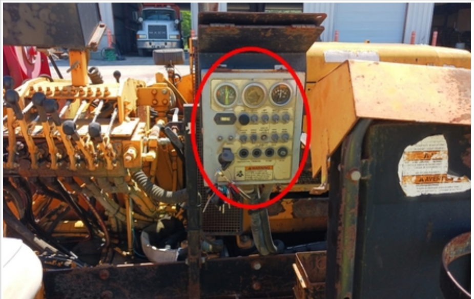
above normal wear on gauges
