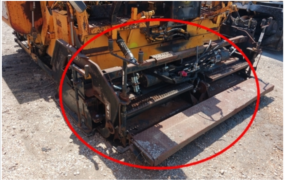
screed shows signs of above wear and tear and is missing 2 burners, so the screed platform does not heat up.
