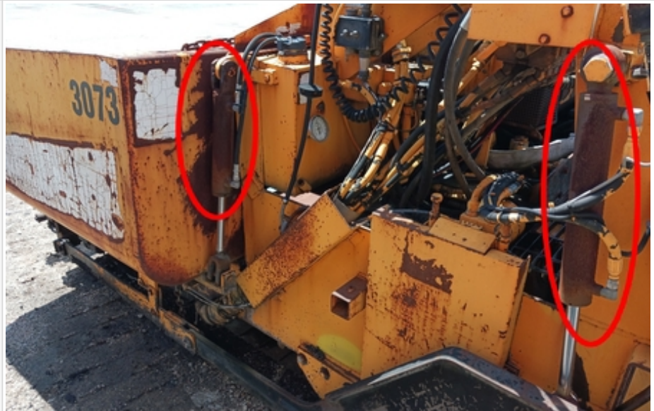
areas of rust on hydraulic cylinders
