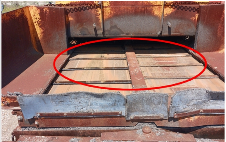
center portion of asphalt hopper has rust
