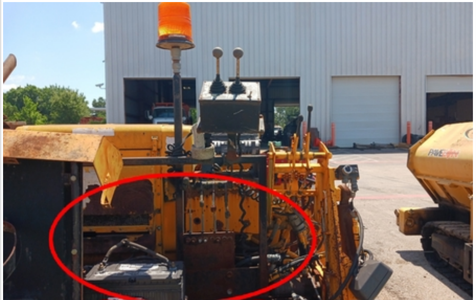
areas of rust
