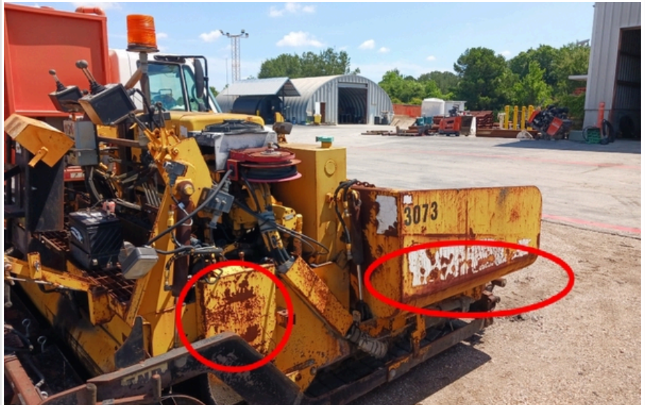
areas of rust
