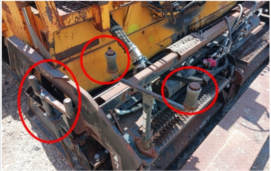
left hand side screed controls have above normal wear and tear
