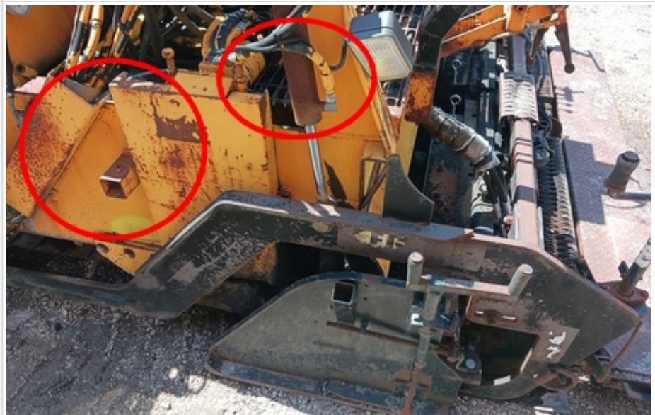
rust on hydraulic cylinder and body
