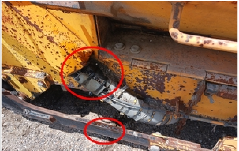
zip ties on hoses and there is a small hydraulic leak
