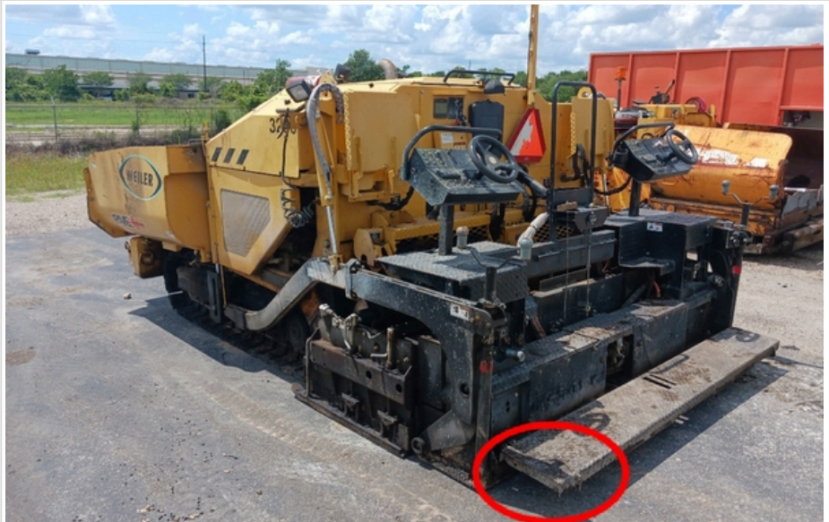
small dent on left hand side screed
