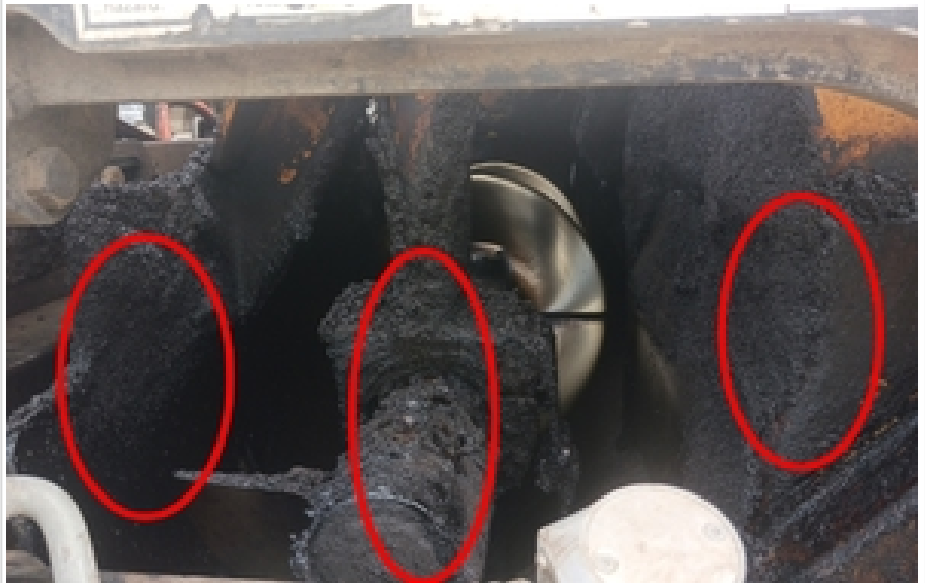
caked up asphalt
