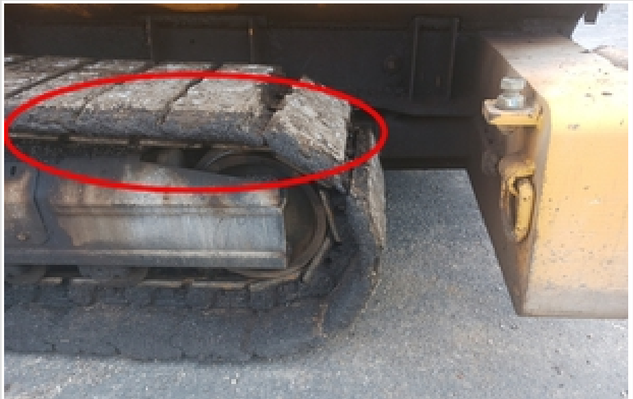
dried asphalt on tracks
