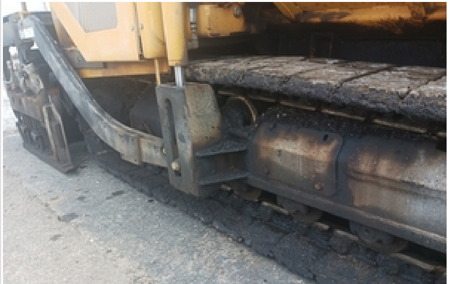
dried asphalt on tracks
