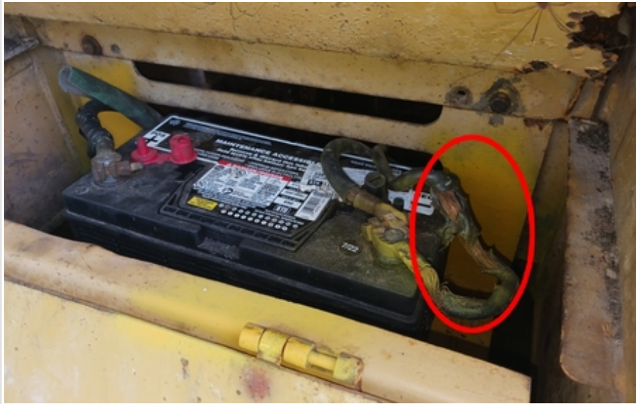
exposed wires on negative battery cable
