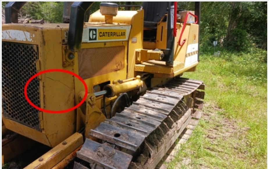
small scratch/missing paint
