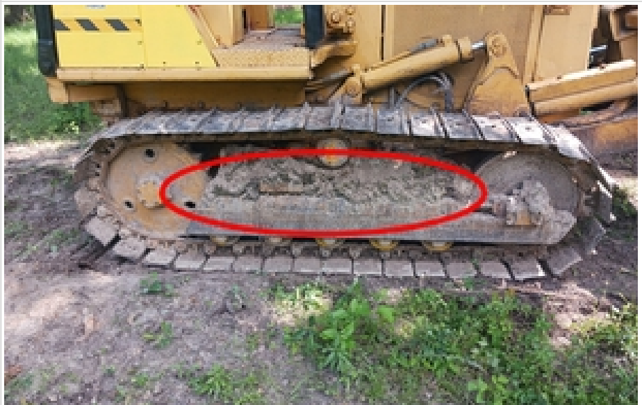
dirt build up
