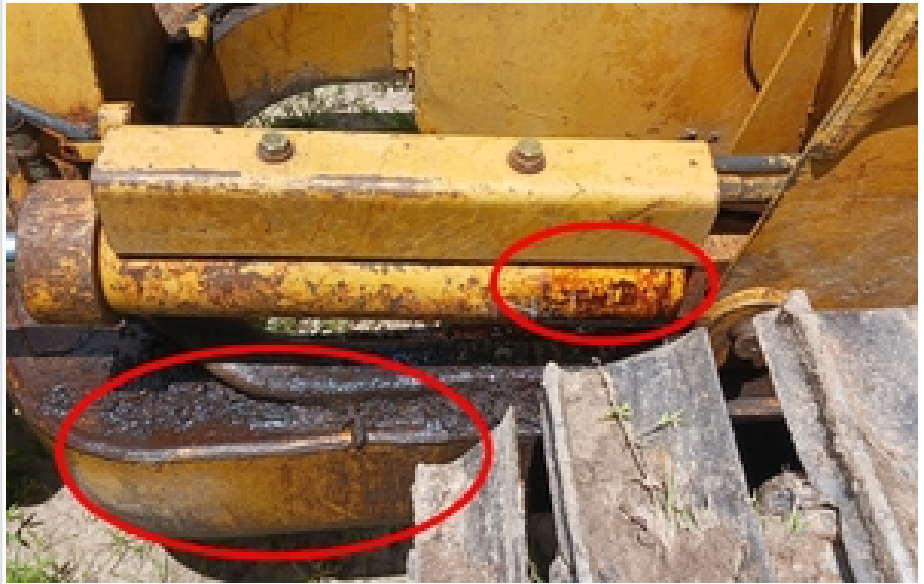
there is a hydraulic leak under the guard
