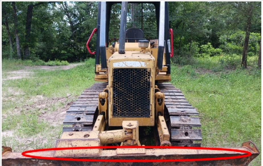
area of rust
