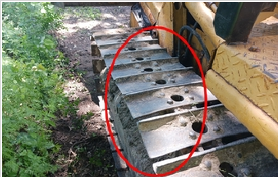
above normal wear and tear on tracks
