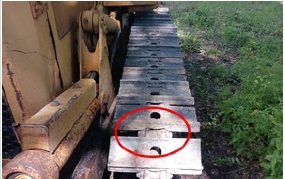
above normal wear and tear on the tracks
