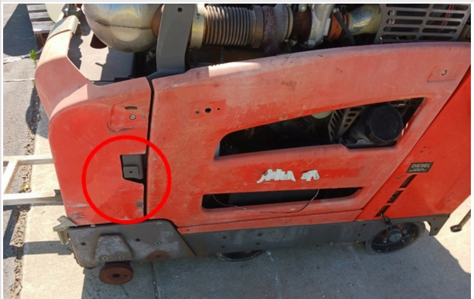
does not latch properly
