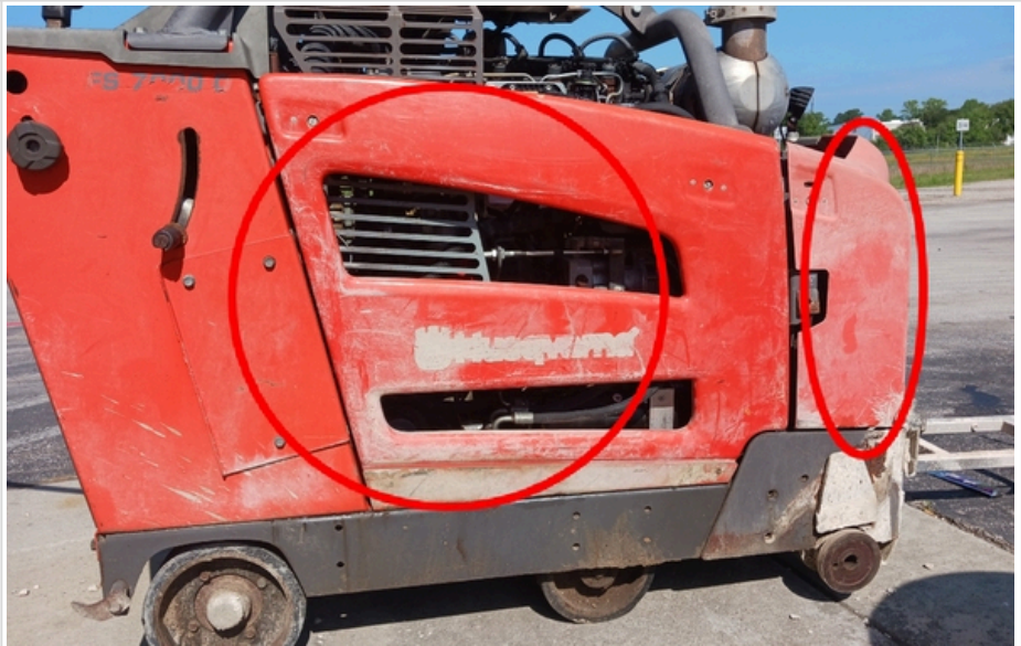
both front and right hand side panels are loose, do not latch properly
