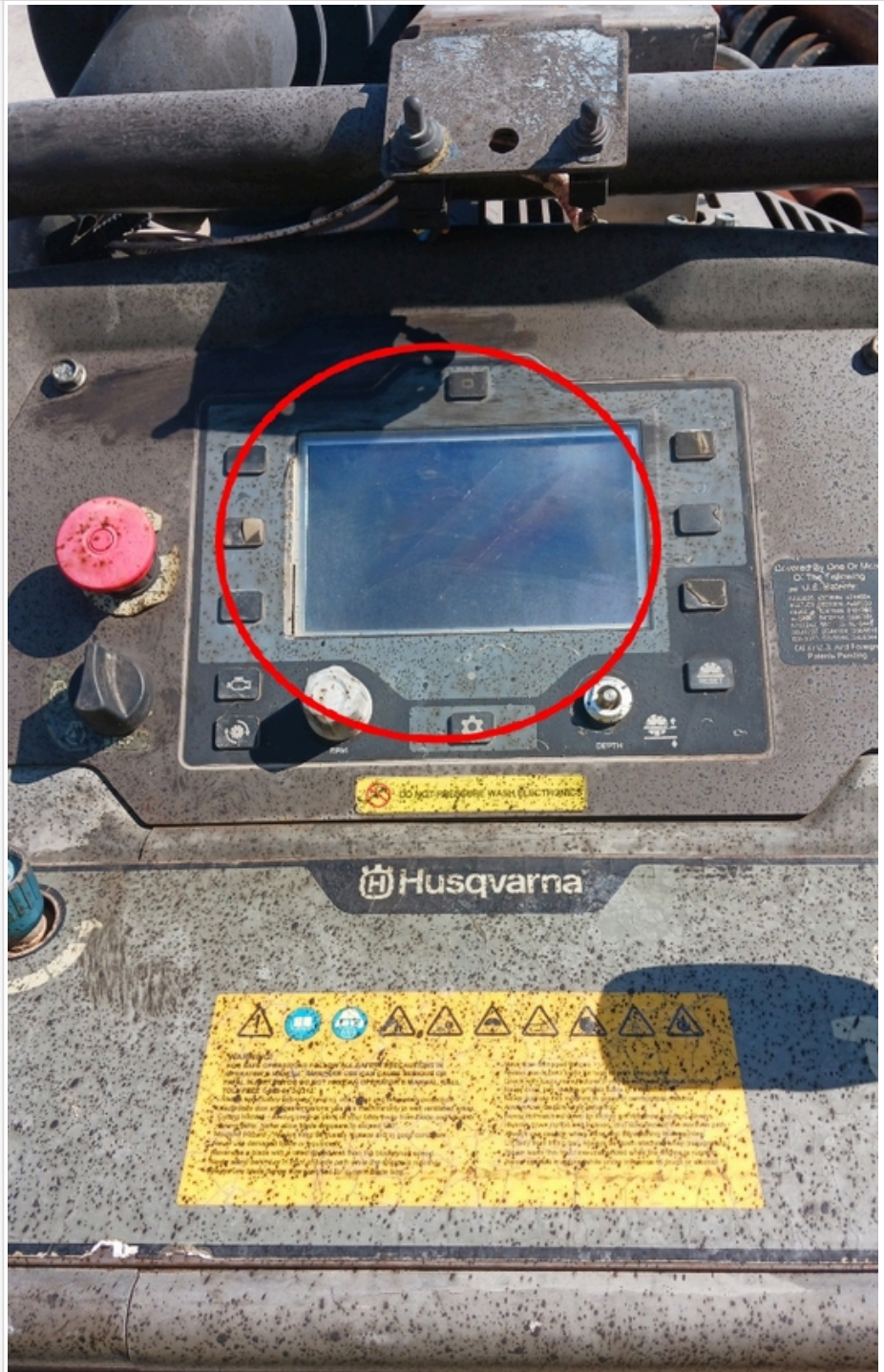
screen does not work and it is cracked
