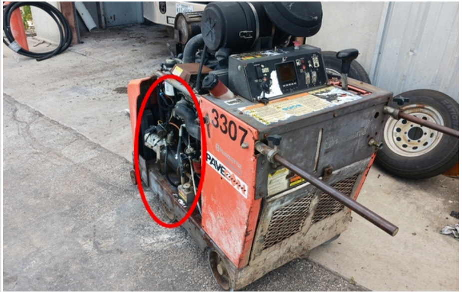
panel is not attached but fits loosely
