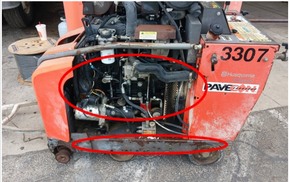
panel not attached but fits loosely when it is. areas of rust
