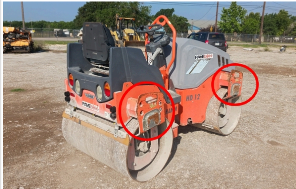
small areas of rust/missing paint
