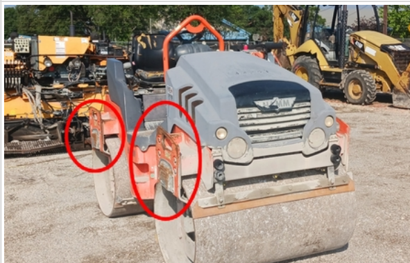
small areas of rust/missing paint
