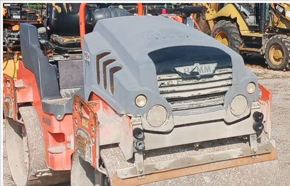
small areas of rust/missing paint
