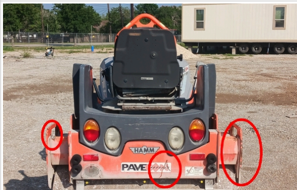
small areas of rust/missing paint
