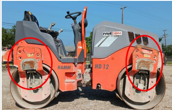
area of rust/missing paint
