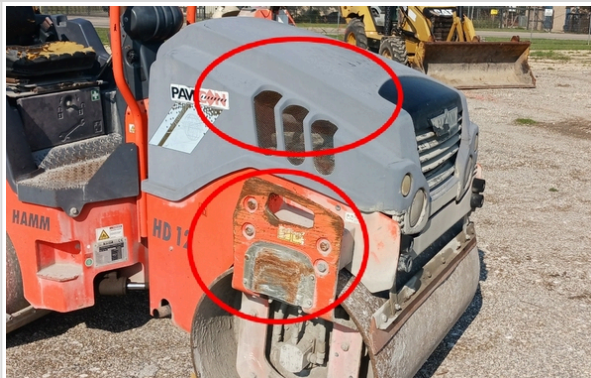
area of rust/missing paint, and faded hood
