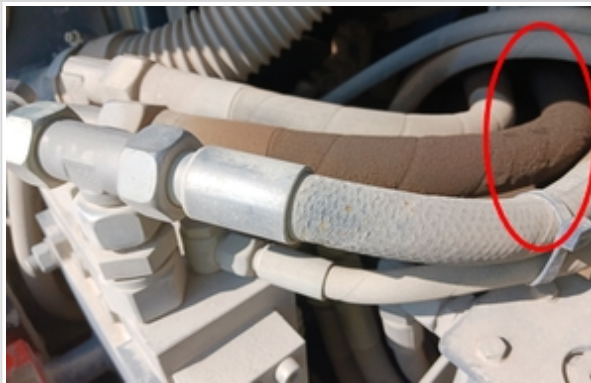
moist area with dirty/gunky residue on the hose
