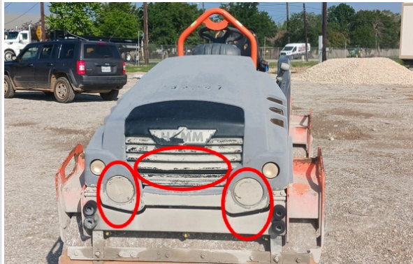
faded/missing paint on grill and the lights are dirty
