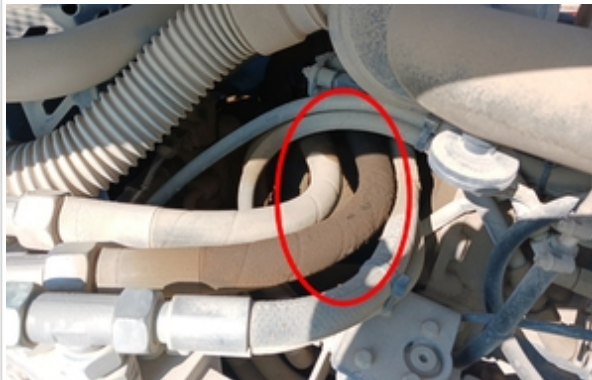
dirty/gunk area and area was moist
