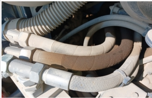
moist area with dirty/gunky residue on the hose
