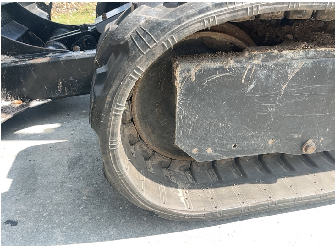
Left Track Condition / 04-04-2024
