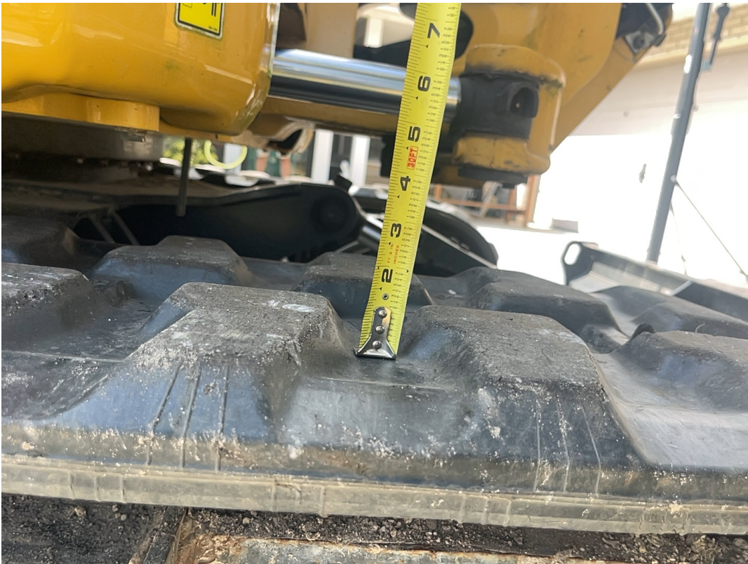
Right Track Tread Depth Measurement / 04-04-2024
