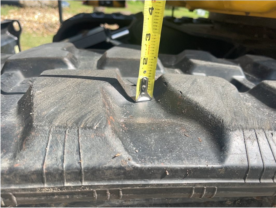
Left Track Tread Depth Measurement / 04-04-2024
