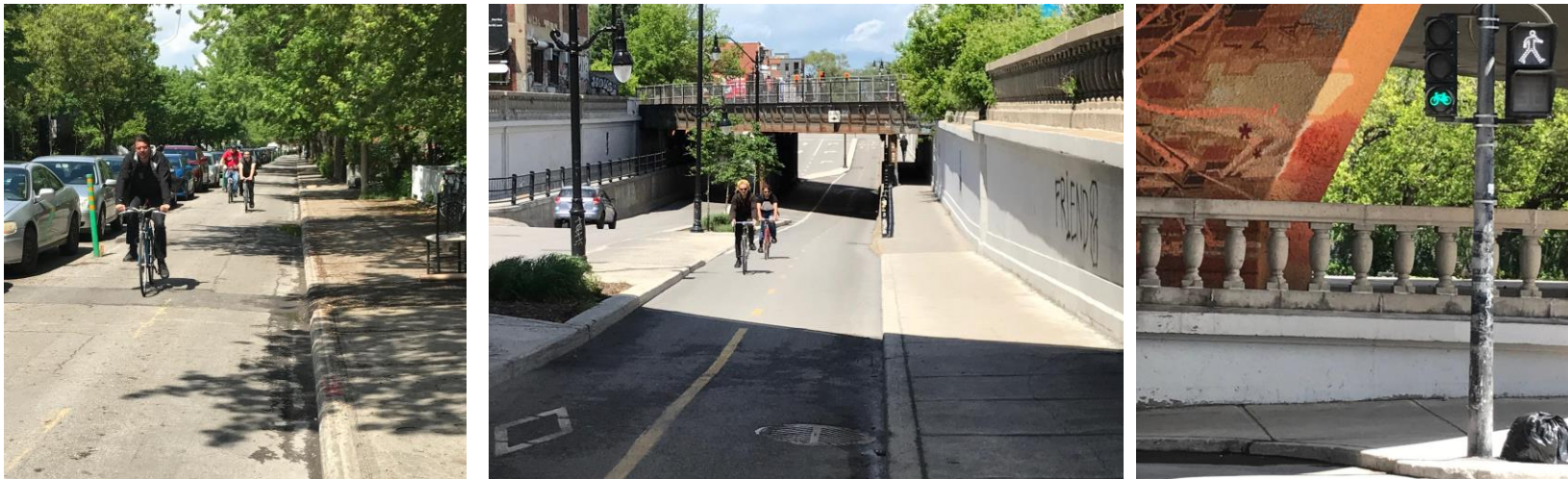
Figure 5: left, parking protected cycling facility (Clark); middle, cycle track at underpass (Saint-Laurent); right, bicycle signal head (Saint-Laurent)
