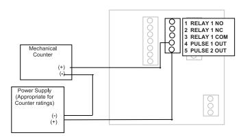
Figure 9: Relay and Switch Wiring Examples
