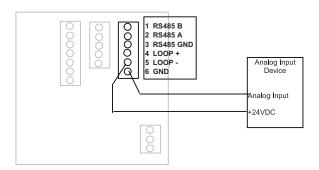
**Figure 13: Current Sinking Analog Output**
