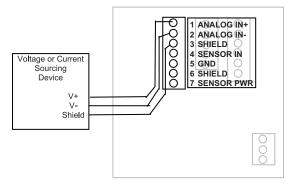
Figure 6: Voltage or Current Sourcing Analog Inputs
