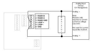
**Figure 12: Current Sourcing Analog Output**
