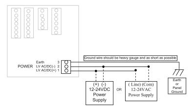
Figure 3: Power Supply Wiring
