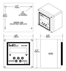
**Figure 2: Wall Mount and Dimensions**
