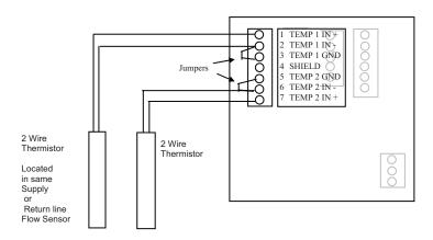
Figure 7: Wiring Two-Wire Thermistors and RTDs
