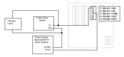
**Figure 10: Relay and Switch Wiring Examples (continued)**Chiller Control Based on High Energy Usage with Indication
