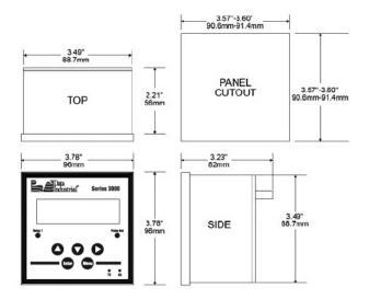
Figure 1: Series 3050 Panel Mount and Mounting Dimensions
