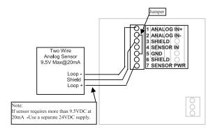
Figure 5: 4-20mA Analog Loop Powered Wiring
