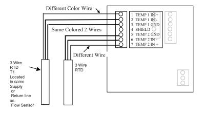
Figure 8: Wiring Three-Wire RTDs
