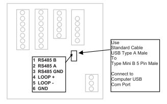
Figure 15: USB Analog Output
