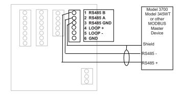
Figure 14: RS485 Communication (Modbus and BACnet)
