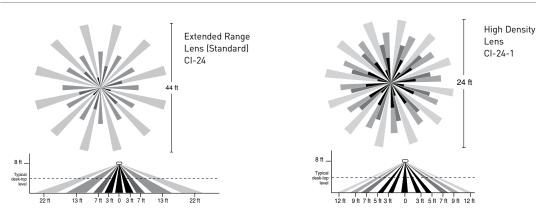
Coverage shown is maximum and represents coverage for half-step walking motion. Under ideal conditions, with no barriers or obstacles, coverage for half-step walking motion can reach up to  $1200 \, \text{ft}^2$  using the Extended Range lens and up to  $500 \, \text{ft}^2$  using the High Density lens. For typical desktop level of activity, coverage can reach up to  $300 \, \text{ft}^2$  using the High Density lens.
