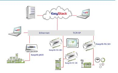
EasyStack is a software technology that combines the core functionality of a Building Automation System (BAS) for connecting and controlling devices, with the added benefits of a Building Operating System (BOS) to manage and leverage data. The technology uses Haystack tagging and data modeling to provide unprecedented capabilities and functionally. The Haystack open standard also provides options and choices for the best combination of solutions from the wider collaborative Haystack community.
