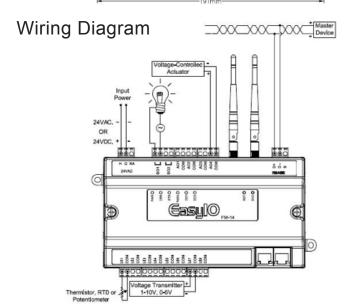
The FW-14 comes with one standard RS485 driver to support BACnet MSTP. The FW-14 also comes with two Ethernet Ports to program the Sedona Application, TCOM, FGP2P, BACnet and for web configurations.
