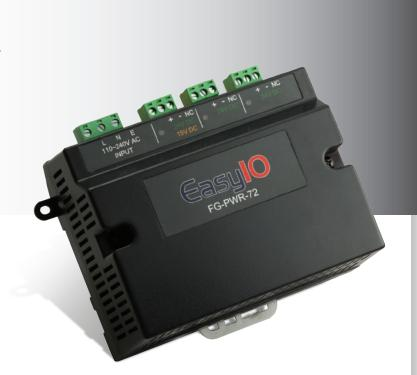
A High quality DIN Rail Mounted isolated 3 x 24VDC, 1 amp each, BMS Power Supply. The first output can also provide 15V DC using a jumper setting.
