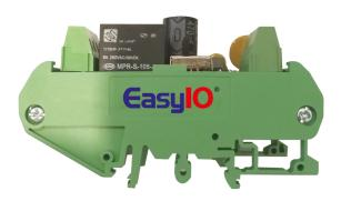
The FR-02 is a relay module which can be mounted on dinrail. It allows 1 x AO coming from a controller to provide floating control via two built-in relays. The modes 1 or 2 are selected by a jumper on the FR-02. Relays rated for 5 million cycles.
