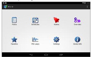
No need for extra programming, the different interfaces are automatically generated from ECLYPSE controllers or EC-Net systems.
