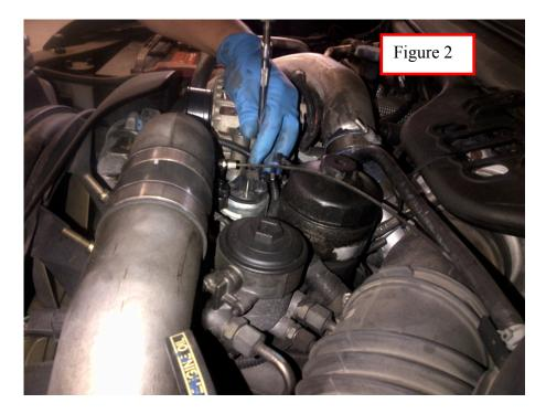
5. Install 201380 adapter (see figure 3) in place of above EGR valve.
