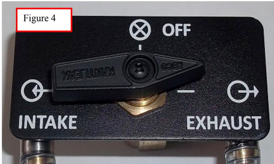
7. Open the air valve, adjust the regulator to maintain the initial pressure, and then open the fluid valve on the EGR Cleaning Tool.
