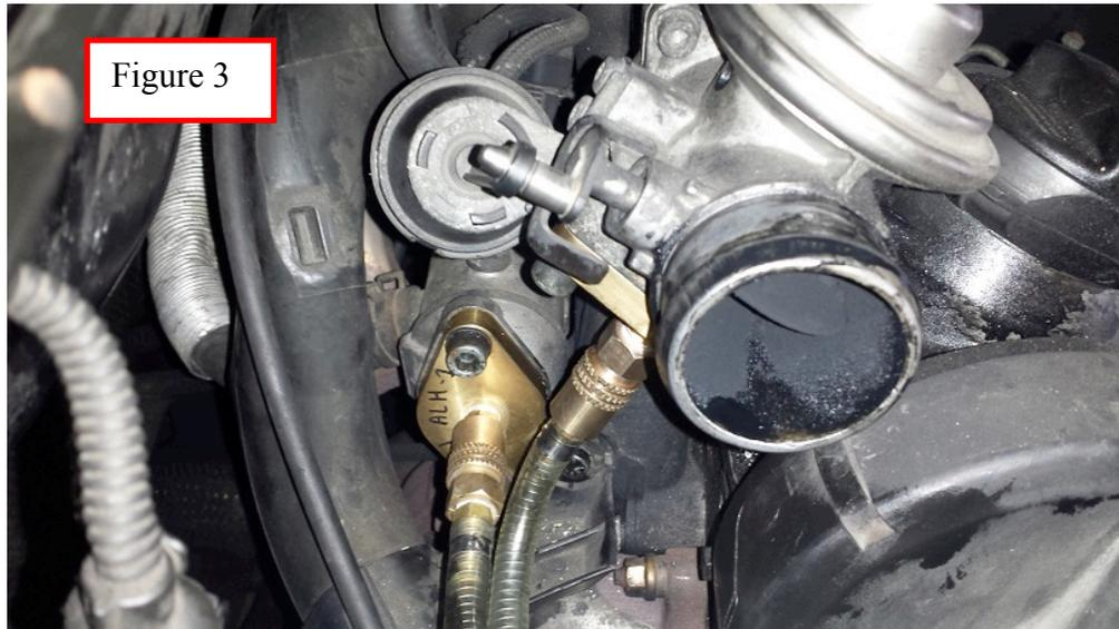
3. Attach the EGR Manifold (201399) to the EGR intake and exhaust adapters. Attach the EGR Cleaning Tool (201170) to EGR Manifold. Ensure air valve and fluid valve are closed – see the EGR cleaning Tool user guide.
