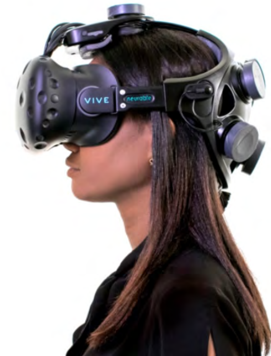
HTC Vive headset with Neurable brain computer interface
