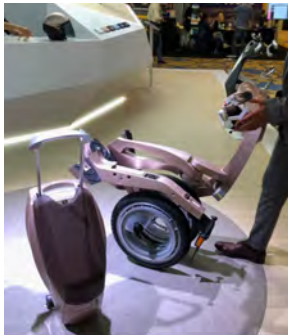
Electric scooter folds for stowing and seat becomes roller case
