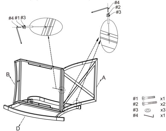
Step 3. Attach right arm panel (part C) to back panel (part A) and seat panel (part B) using bolts (part #1), long bolts (part #2), flat washers (part #3) and allen wrench (part #4).
