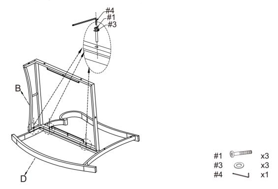
Step 2. Attach back panel (part A) to left arm panel (part D) and seat panel (part B) using bolt (part #1), long bolts (part #2), flat washers (part #3) and allen wrench (part #4).
