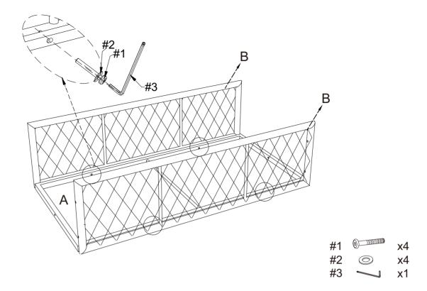
Step 2. Attach end panels (part C) to top panel (part A) and side panels (part B) using bolts (part #1), flat washers (part #2) and allen wrench (part #3).
