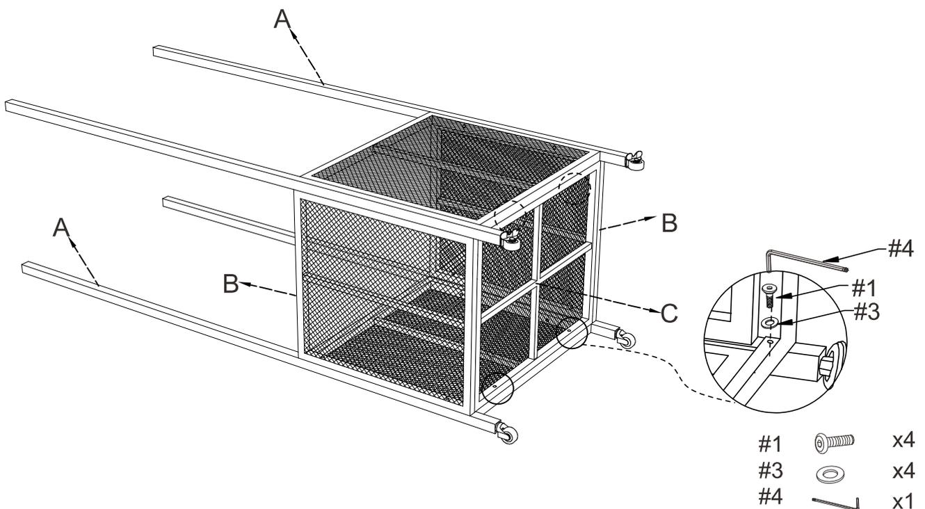
Step 5. Attach shelf (part C) to long side panels (part A) using bolts (part #1), flat washers (part #3) and allen wrench (part #4).
