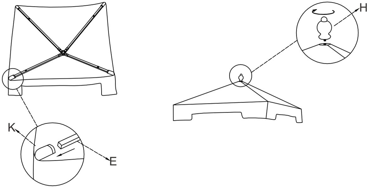
Step 10. Attach assembled unit (parts E, F, H & K) to connectors (part G) using bolts (part #1), flat washers (part #3) and allen wrench (part #4).
