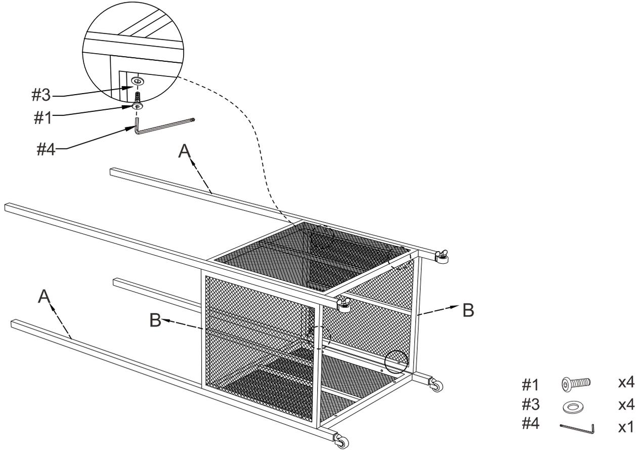
Step 4. Attach bottom panel (part C) to long side panels (part A) and short side panels (part B) using bolts (part #1), flat washers (part #3) and allen wrench (part #4).
