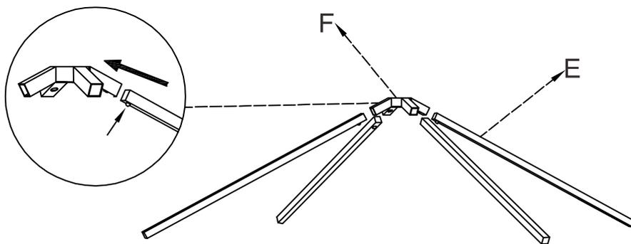
Step 9. Unfold top cover (part K) and attach to assembled unit (parts E & F) as shown below.
