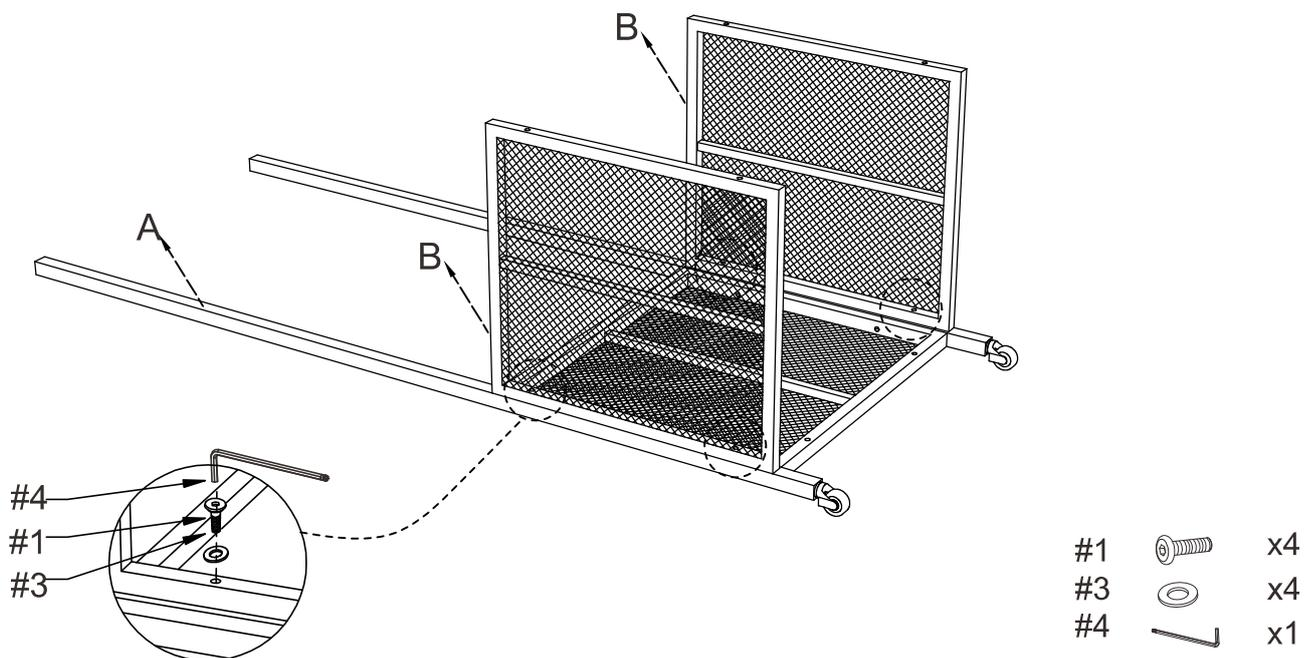
Step 3. Attach long side panel (part A) to short side panels (part B) using bolts (part #1), flat washers (part #3) and allen wrench (part #4).
