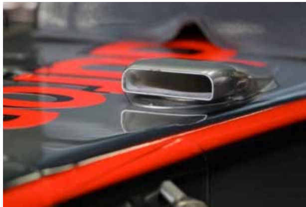
The F-Duct on the 2010 McLaren MP4/25
