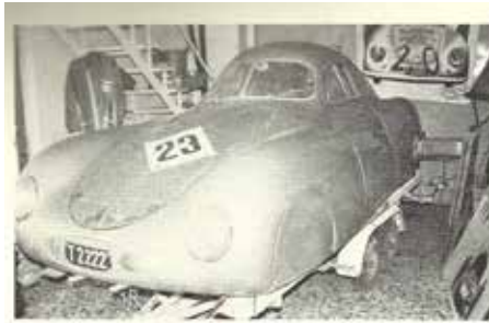
The Type 60K10 that Mathe' owns. This is the car that Professor Porsche used during the war. The car has been repainted, wipers placed below the windshield and controls transferred to the right side by Mathe' who lost his right arm in a motorcycle accident in 1934. The body is very light, and made of aluminum.
