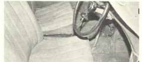
The twin seats of the 60K10. Mathe' converted the car to right hand drive. He also changed the brakes from cable to hydraulic. Mathe' shifts by pressing his shoulder to the wheel and then shifting with his good left hand.
