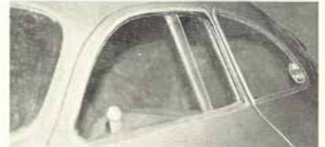
The side window detail of the 60K10. The windows are flush and the doors fit close. A rollup window would require a recessed area, as would rain gutters. The front window slides open.
