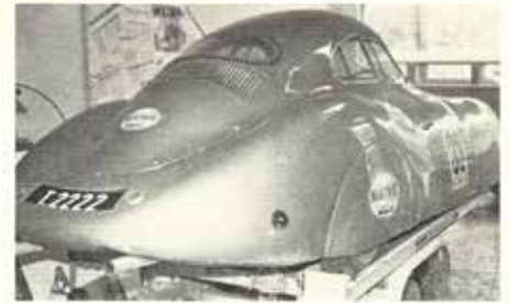
The rear of the 60K10 showing the Jaray lines with a minimum of protuberances. The rear grillwork is right off the Volkswagen, as is the rear window.
