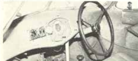
The dash board of the 60K10. A single instrument in the center contains the speedometer and odometer. Mathe' added the watches. 24
