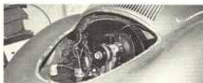
The engine compartment of the 60K10. The lid is removed by Zeuss-type fittings. The engine is not the original unit.
