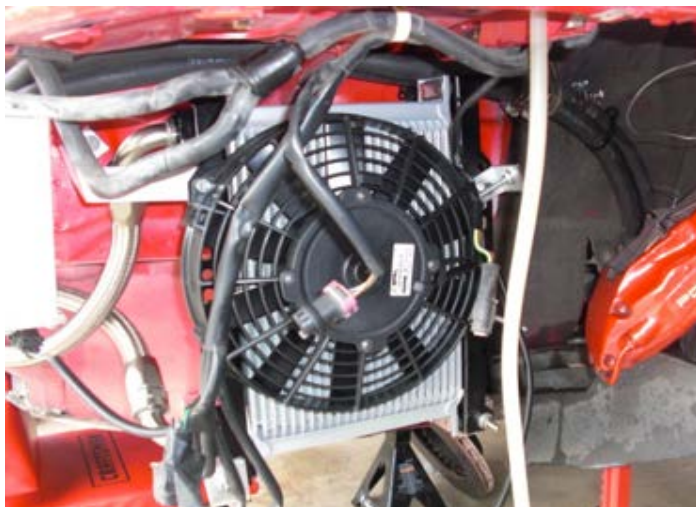
BAT Oil cooler solved hot running issue
