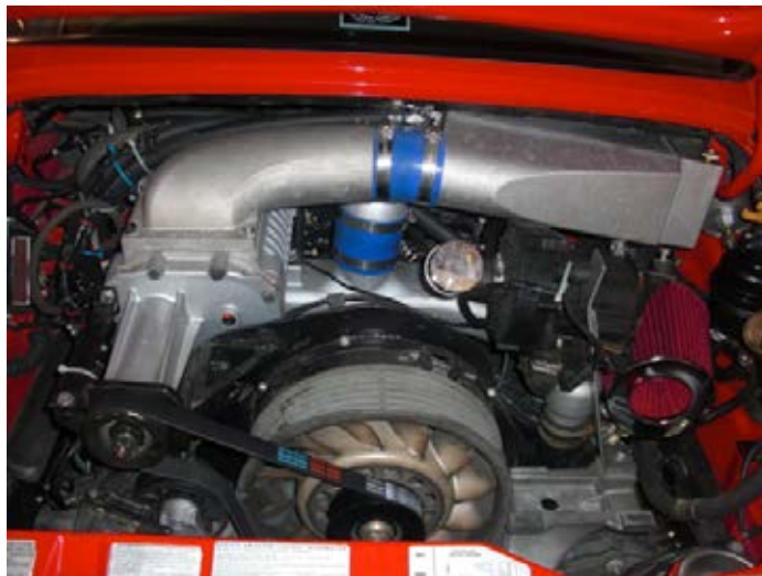
Completed Supercharger installation Thanks .. Dart
