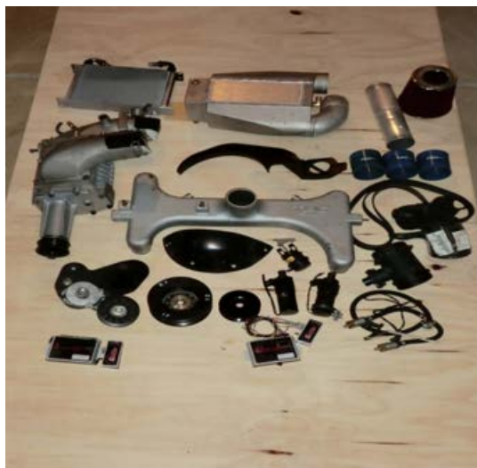
Major Supercharging Components
