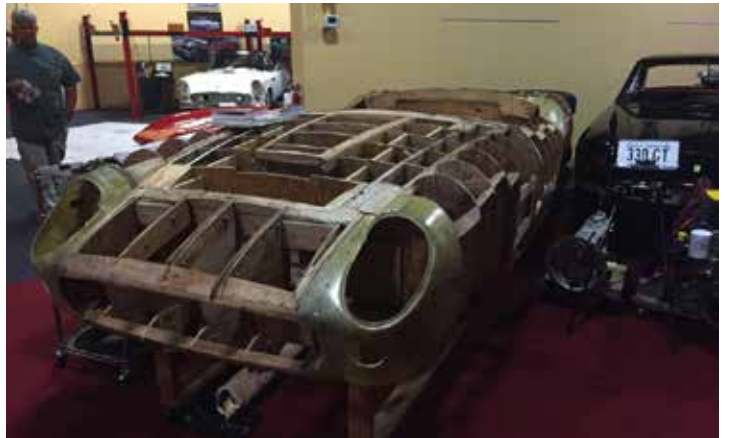
It was now time to visit the fab shop. Oh by the way, Oscar and Evan are now creating a 1960 Ferrari California Spyder, based on a 1962 330 GT. Creating body panels will prove to be a slightly simpler task as the collection sourced and bought a wooden body buck used to create the original 250 California Spyder.
