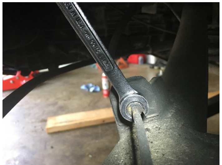
Figure 2: flare nut wrench on brake fitting
