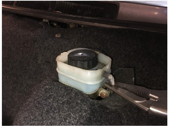
Figure 3: Brake fluid reservoir with overflow clamped
