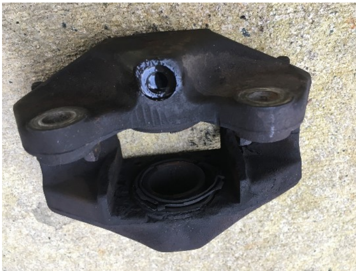
Figure 1: Caliper with disintegrated seal
