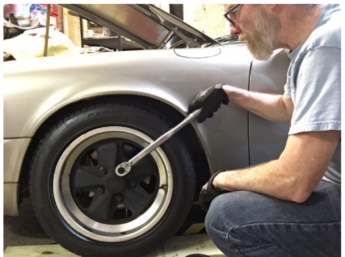
Figure 4: torquing with shiny new lug nuts
