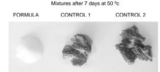
All Mixtures were placed in airtight packages and stored in a chamber pre-heated to 50 °C. After 7 days, packages were opened and the appearance of formulations checked. The results showed the improved stability of Formula, which can tolerate storage at higher temperatures without suffering deterioration.
