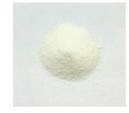
**FORMULA** was introduced into an airtight package and stored at 25 °C. After 18 months the pack has been opened and the appearance of formulation checked. The formulation still looks white, without aggregates, and flows freely. Results show long term stability of FORMULA which does not suffer any alteration after 18 months when stored at room temperature.
