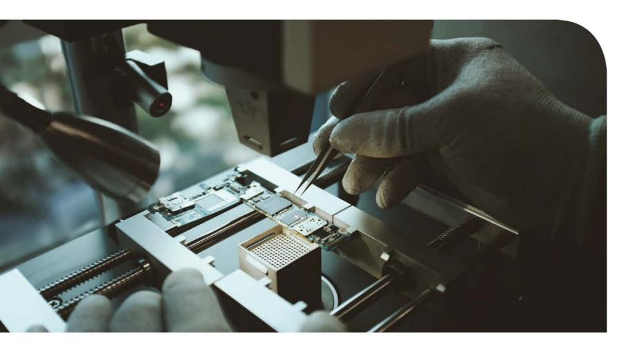
MD-MR is the package of hardware devices to detach the memory from the board of mobile phone or digital device. When the device is severely broken, burnt, or drowned, MD-MR is used to prior to Chip-off forensics. MD-MR includes 5 flash memory sockets for MD-READER, heat blower, soldering station, fume extractor, microscope with optional components of mobile device dryer, rework system and mobile device safety box.
