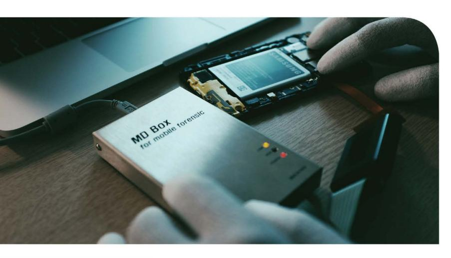
MD-BOX is the forensic hardware for extracting data directly from the mainboard using JTAG interface. When the mobile device has damage on the external parts, but the mainboard still works, the examiner can connect the mainboard to MD-BOX through JTAG interface. Then, the data can be extracted at the menu of JTAG Extraction in MD-NEXT program.
