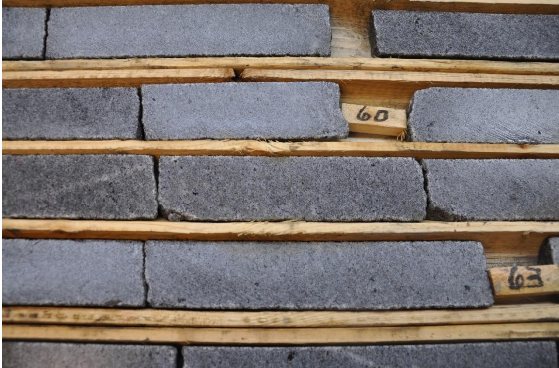
Figure 7.4 – Low-Grade (LG) Zone observed in the Graphene-Battery Zone in drill hole LL-14-05 (from 58.0 to 64.0 m)
