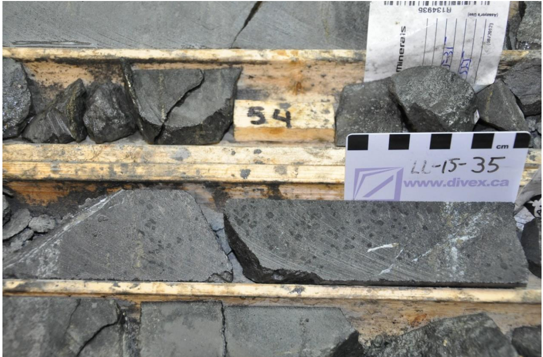
Figure 7.5 – High-Grade (HG) Zone in the Graphene-Battery Zone in drill hole LL-15-35 (54.0–58.0 m). The core shows the dark porphyroblasts associated with HG zones.
