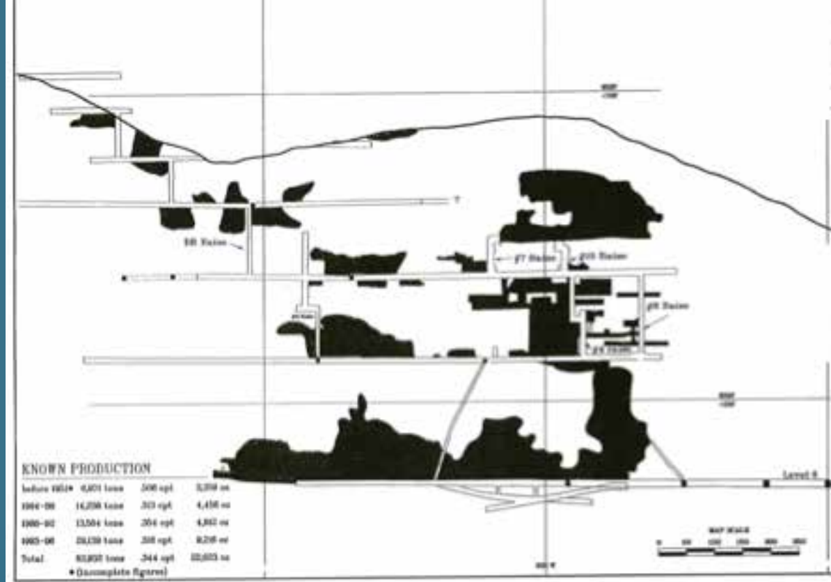
Long section showing underground development in Gold Prince Mine
